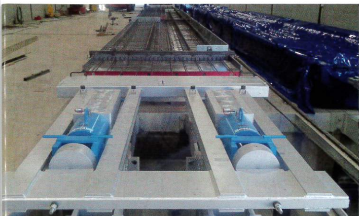
Production lines Detensioning side
