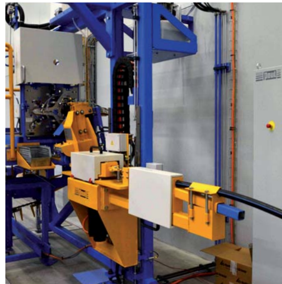
Fig. 3: Button heading and checking unit (stationary), Wire feeding and cutting unit (moving)
