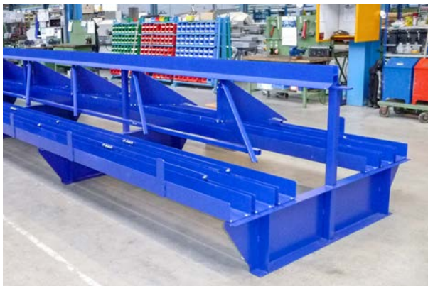
Pushing channel with 3 trays on the right, 3 trays on the left
