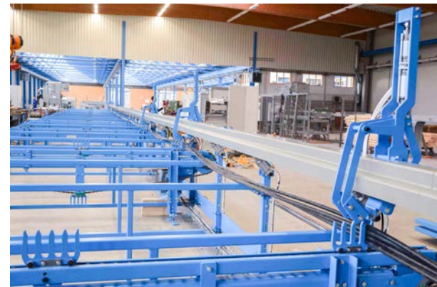
Anchor manufacturing with strand tray arranged in 4 rakes by pneumatic actuating cylinders for 3 anchors, cross transport with chain
