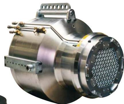
Fig. 5: 12500 kN stressing jack, stroke 200 mm, for 91 x 0.6"
