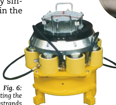
Fig. 5: 12500 kN stressing jack, stroke 200 mm, for 91 x 0.6"
