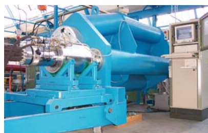
Fig. 7: On the PAUL stressing jack test stand it is possible to determine the friction of your stressing jack up to 3000 kN (10000 kN), e.g. of the PAUL TENSAM 3000 kN jack according to accuracy class 0.5 to DIN 7500-1.
