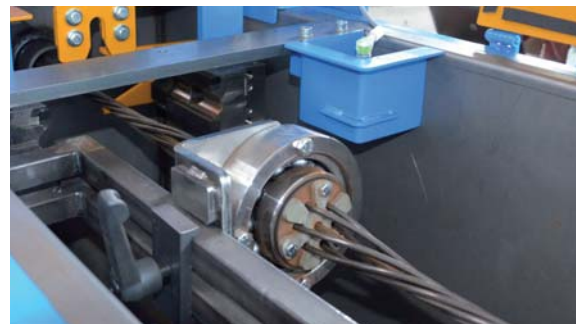
Fig. 2: Greasing the strand
